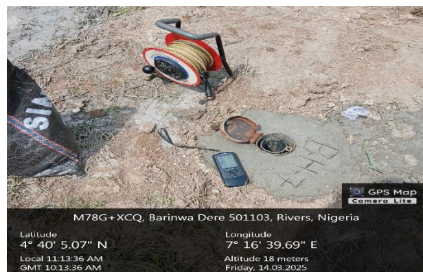
Groundwater investigation using oil-water interface meter.
